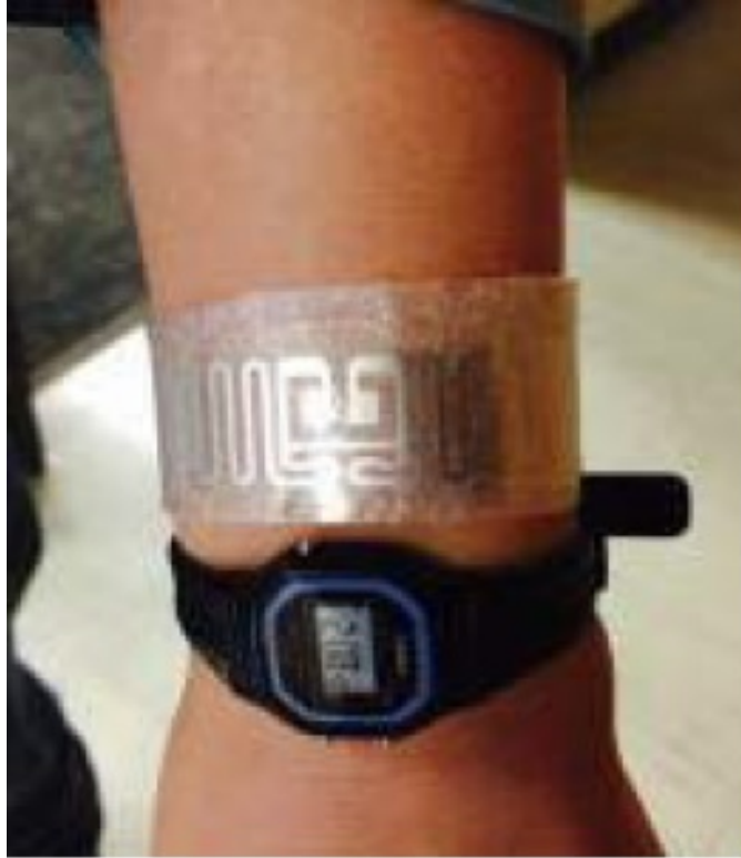
Figure 2.1: Flexible Circuit: Flexible Wireless Temperature Sensor System [1].
