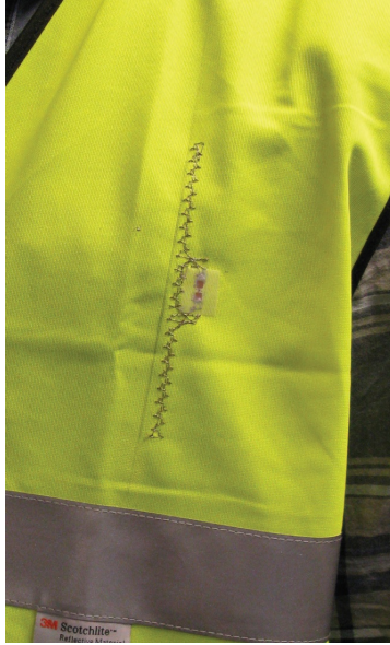
Figure 2.3: Flexible Antenna Printed on a Fabric Substrate [4].
