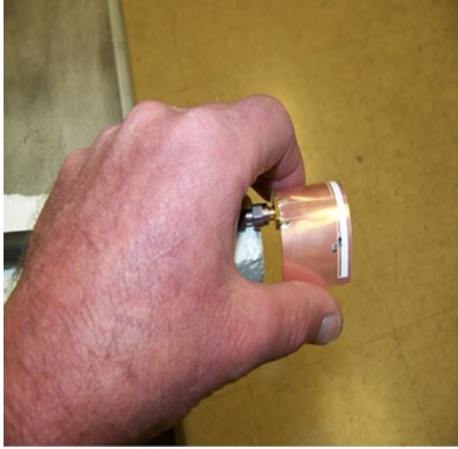
Figure 2.2: The Proposed Flexible Folded Slot Antenna Printed on PET Material.
