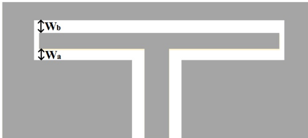
Figure 2.26: Symmetrical CPW-Fed Folded Slot Antenna.
