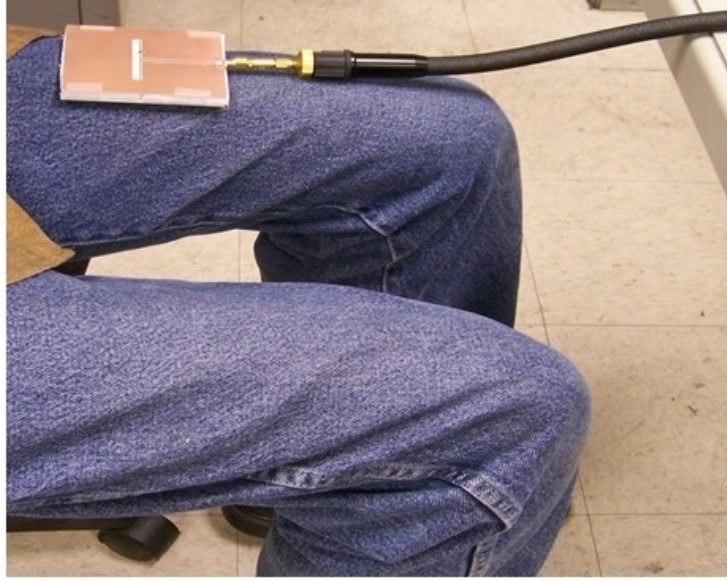
Figure 4.15: Fabricated Prototype of the Antenna Structure Placed on Human Body.
