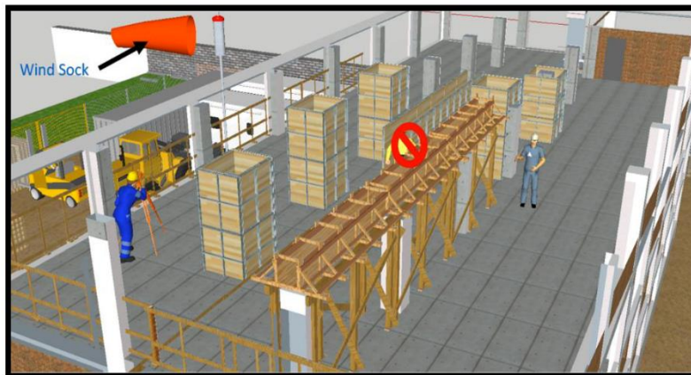
Figure 20. Formwork placement and high wind speed
