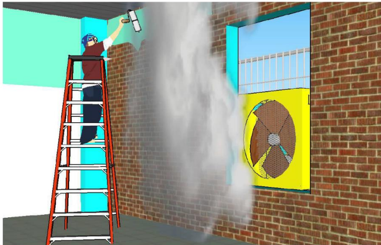
Figure 14. Ventilation installed to remove toxins from the air
