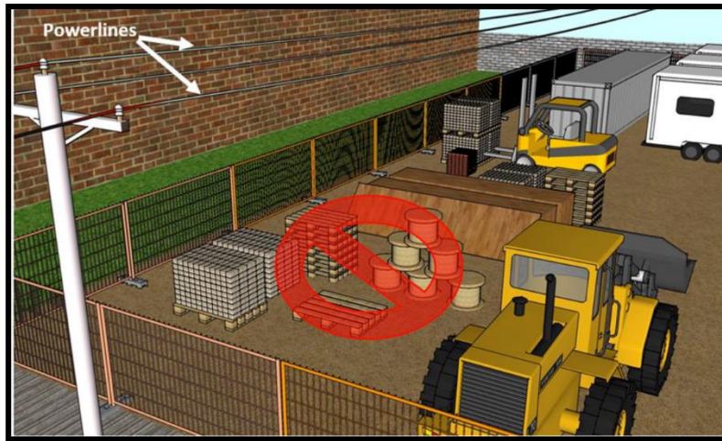
Figure 8. No material storage adjacent to power lines
