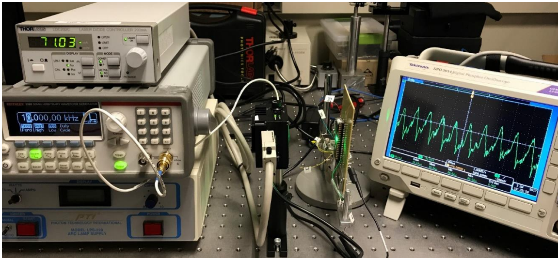
Figure 50. Self-powered Chip for VLC Test Setup
