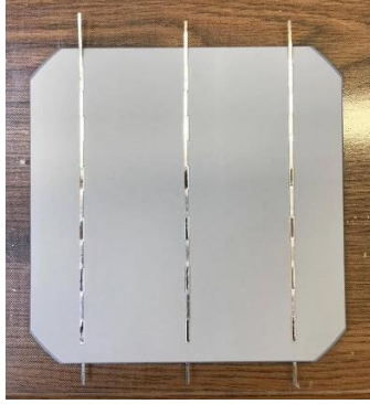
Figure 4 Rear side of soldered cell
