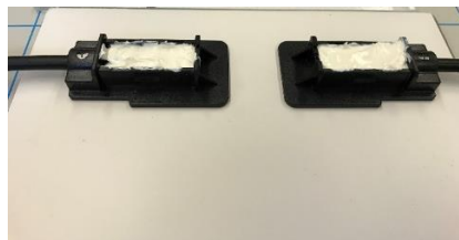
Figure 14 Junction box cavity filled with sealant (glass-polymer coupon)
