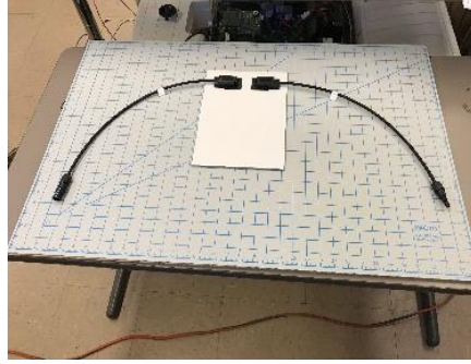
Figure 17 Rear view of glass - polymer coupon with Junction box and connectors
