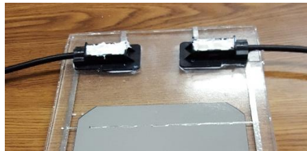
Figure 13 Junction box cavity filled with sealant (glass-glass coupon)
