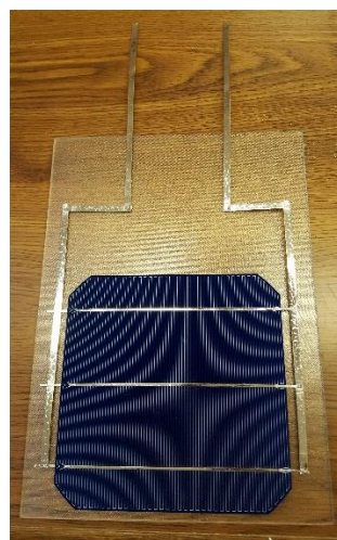
Figure 6 Soldered cell for glass-glass Coupon
