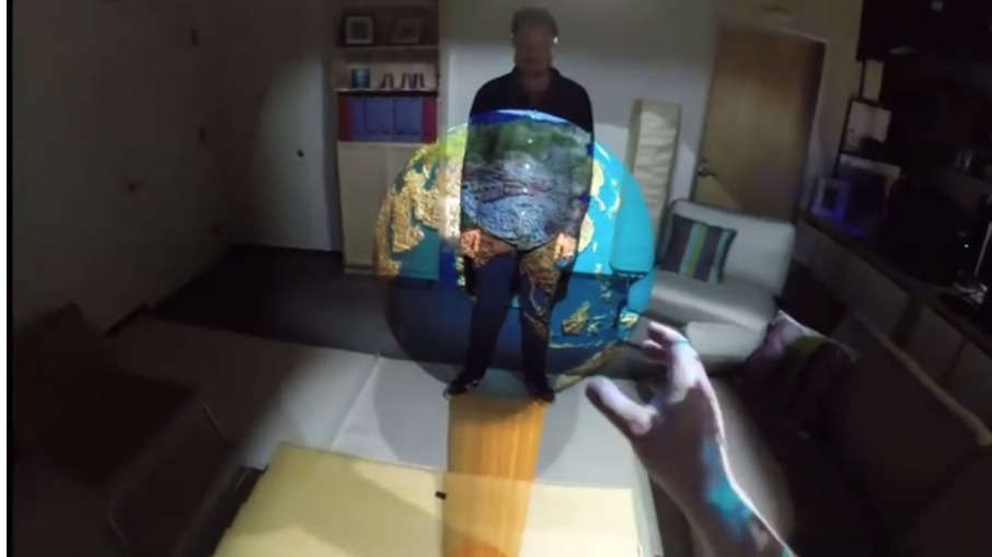
Figure 2.3: Mano-A-Mano, Enabling Two Users To Interact With 3D Virtual Objects Simultaneously (Hrvoje and Andrew et al. 2014)
