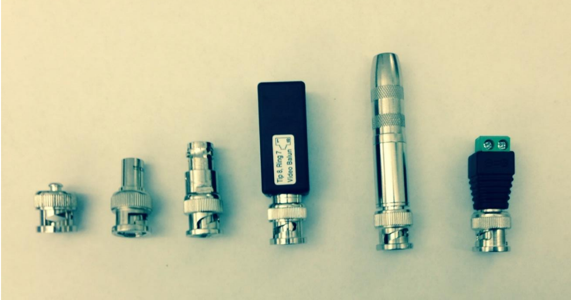
Figure 6: Photo of terminations and adapters used - From left to right, there is the open BNC termination, the 50 \Omega BNC termination, the BNC to triax adapter, the BNC to ethernet adapter, the BNC to audio adapter, and the BNC to two wire adapter, which was used for the twisted pair cable.
