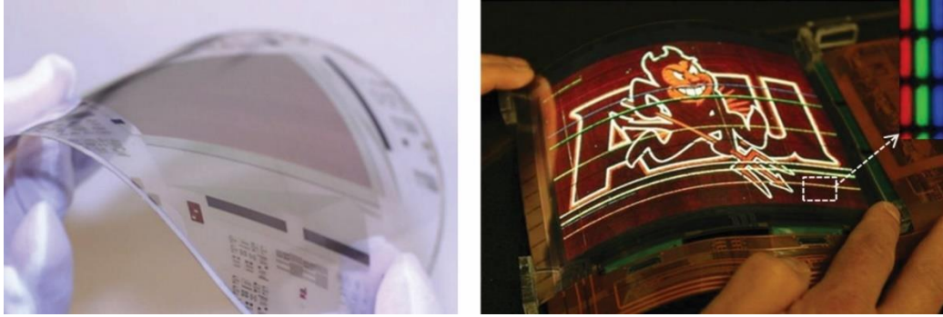
Figure 40: Photographs of a wafer of flexible electronics (left) and a flexible display (right) built at FEDC.
