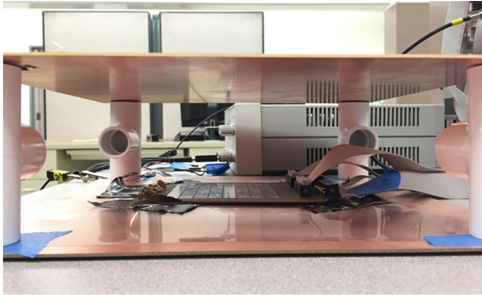
Figure 61: Side-view of testing apparatus. The two large parallel plates create a uniform electric field which is read by the two-dimensional imager. Objects can then be placed between the imaging array and the top plate.
