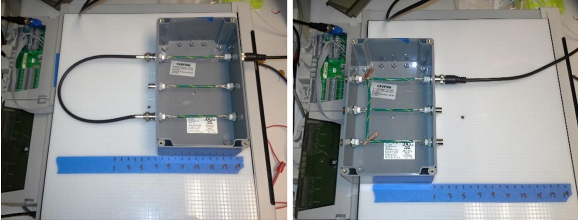
Figure 45: Setup 1: Experimental setup of a plastic box with 3 parallel wires (left). Setup 2: Similar setup but in which the top and bottom wires are connected with a jumper wire within the box (right).
