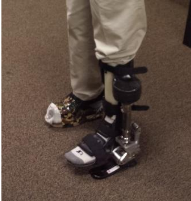
FIGURE 3.14: ANKLE BYPASS SYSTEM TESTING WITH 73KG USER.
