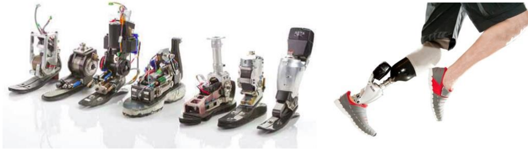
FIGURE 2.7: HERR DEVELOPED A SERIES OF PROTOTYPE ANKLES THAT USED A SERIES ELASTIC ACTUATOR WITH AN ADDITIONAL SPRING IN PARALLEL TO THE LOAD PATH. THE ANKLE WAS COMMERCIALIZED UNDER THE BIONX BRAND, COURTESY OF WWW.BIONX.COM.
