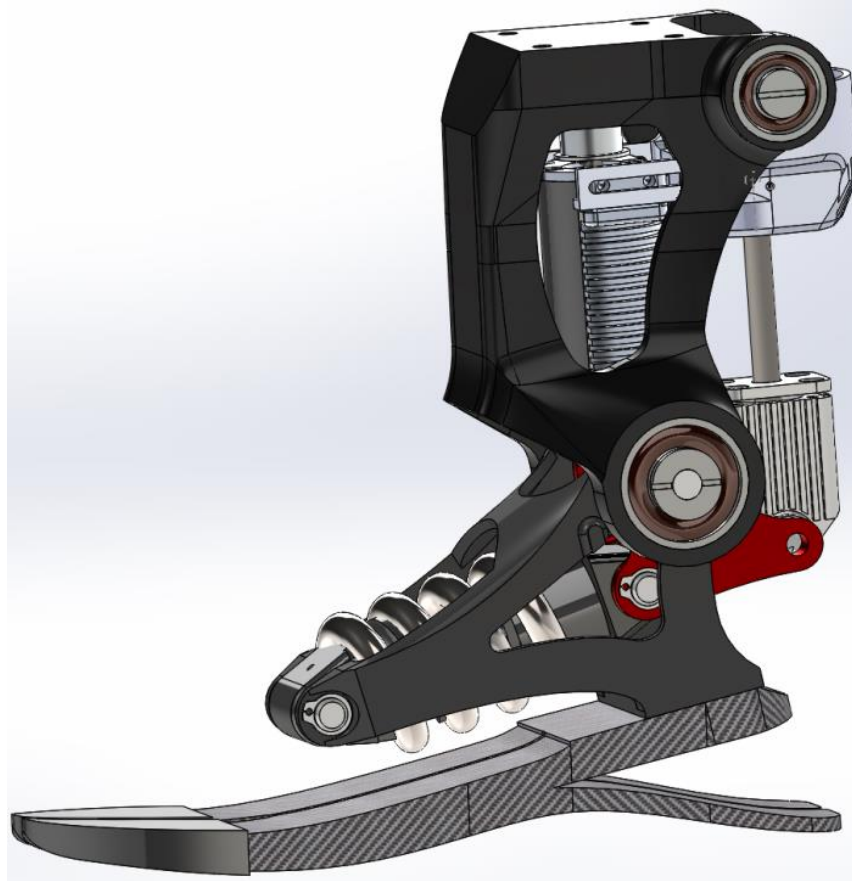
FIGURE 4.6: ASSEMBLY OF ROBOTIC FOOT ACTUATOR SYSTEM
