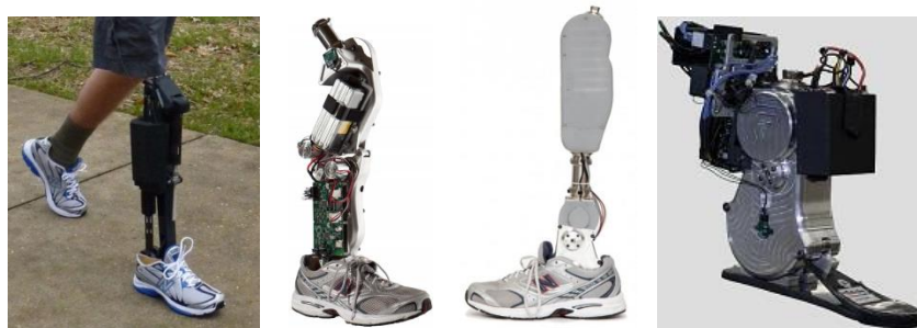
FIGURE 2.9: A TRANS-FEMORAL PROSTHESIS WAS DEVELOPED THAT POWERED BOTH THE ANKLE AND KNEE. CURRENT RESEARCH HAS FOCUSED ON AN ANKLE DEVICE AS WELL.
