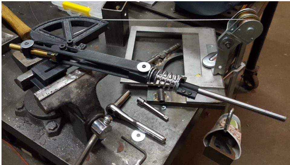
FIGURE 6.23: CONSTANT MOMENT MECHANISM VERSION 1.0.
