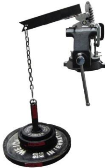
FIGURE 3.13: LEAF MECHANISM TORQUE TEST SETUP.
