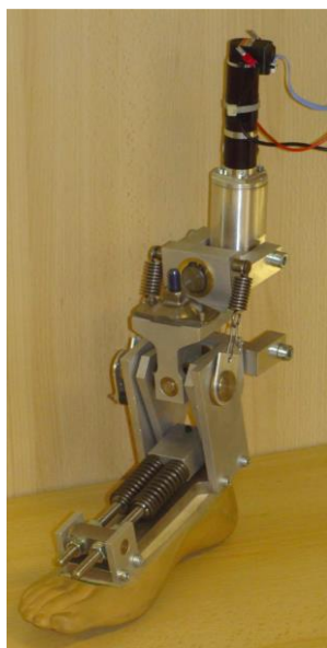
FIGURE 2.12: A SPRING BASED ANKLE WAS CONTROLLED USING ADAPTIVE OSCILLATORS.
