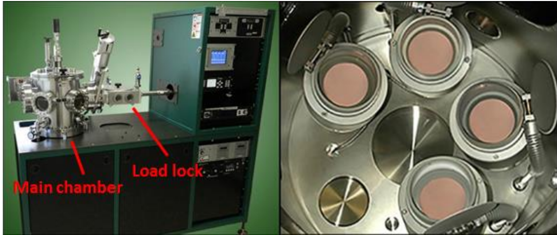
Figure 4: Left: Orion 5 Sputter Deposition Tool used to synthesize metallic and amorphous thin films. Right: Magneton sputtering guns having copper targets. Pictures courtesy AJA International.
