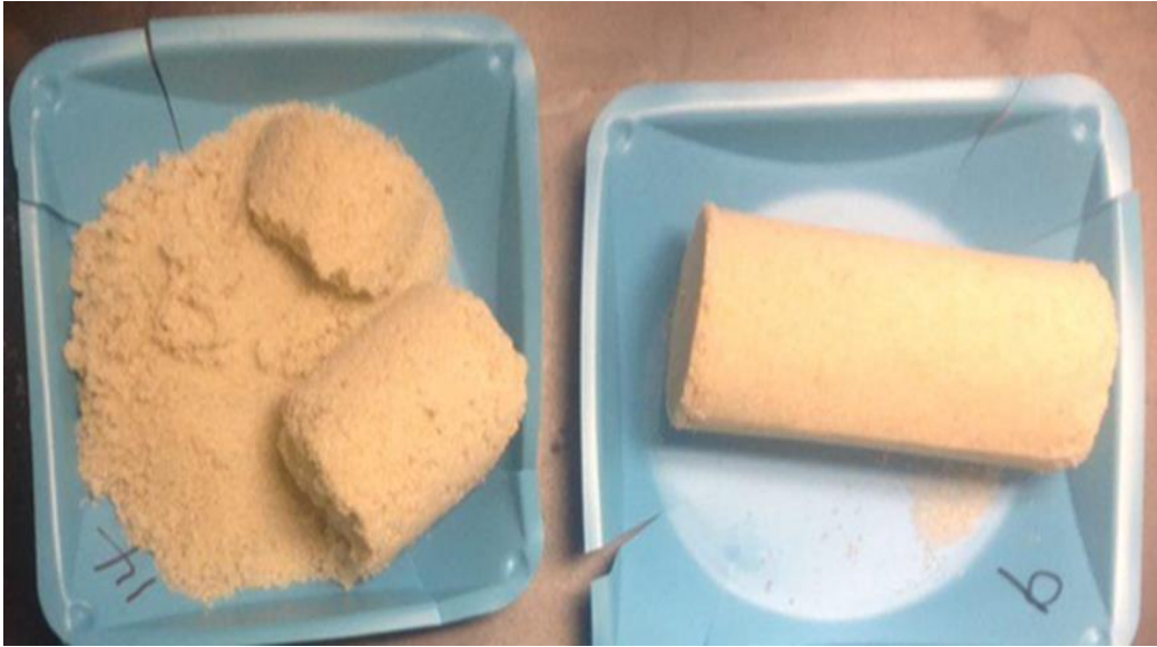
Figure 9. EICP-treated samples by using mix-and-compact (left) and percolation (right) methods.
