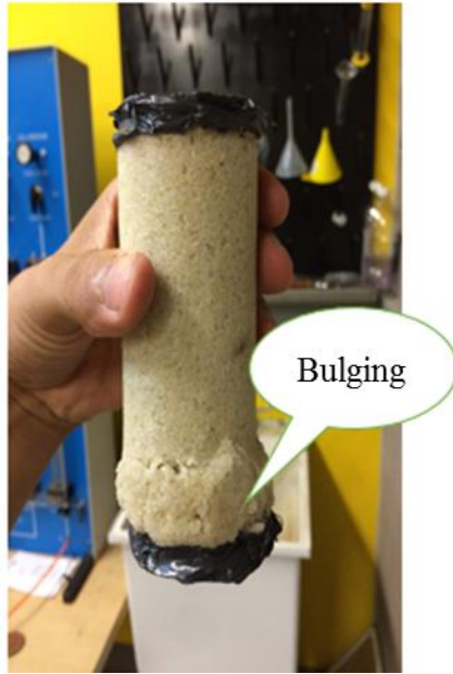
Figure 20. Bulging failure when xanthan gum used as part of EICP solution
