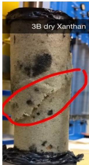
Figure 16: Shear plane for specimen 3B
