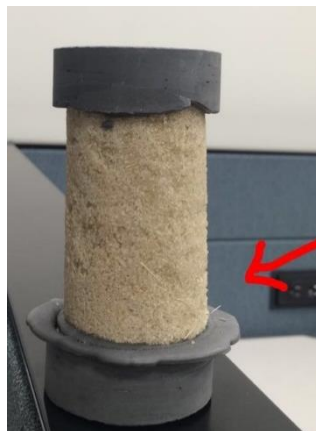
Figure 25: Sisal Fiber Column Prepared for UCS Testing
