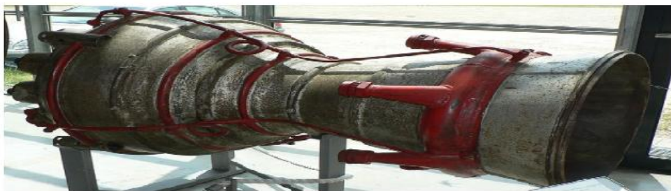
Figure 1.2. Bell Nozzle (courtesy
