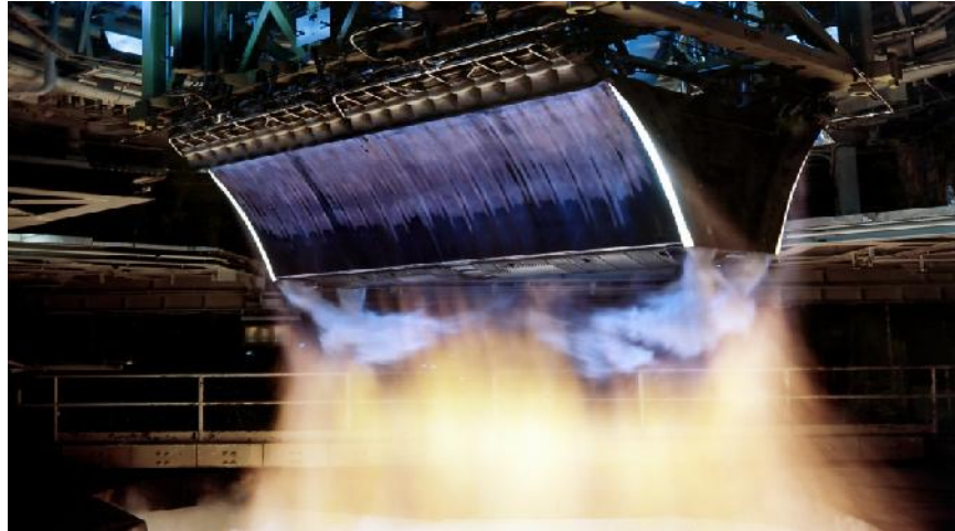
Figure 1.6. XRS-2200 Being Tested for the X-33 Reusable Launch Vehicle
