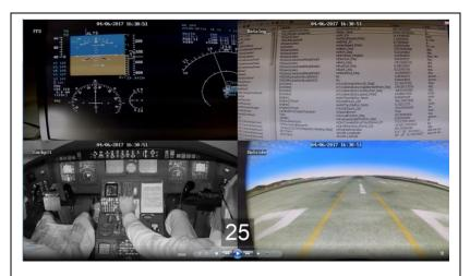
Figure 11 CRJ-200 observation video recording demonstrating the cockpit, PFD, datalogger and external views
