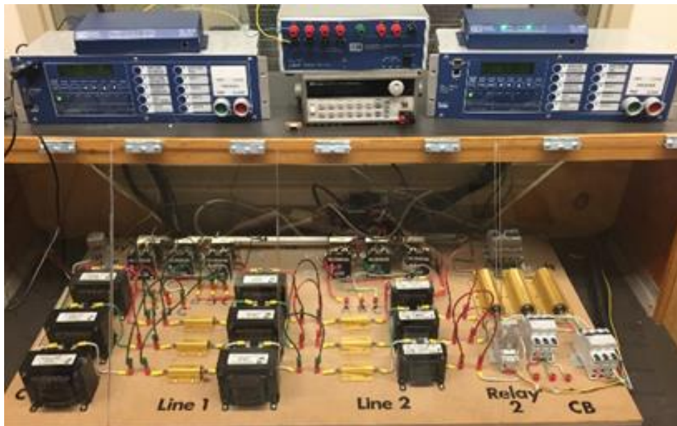
Fig 4.7. Laboratory Setup of Power System Protection with Digital Relays
