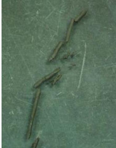
FIGURE 3.2: Crumbled Thread of Anthem Clay in Plastic Limit Test
