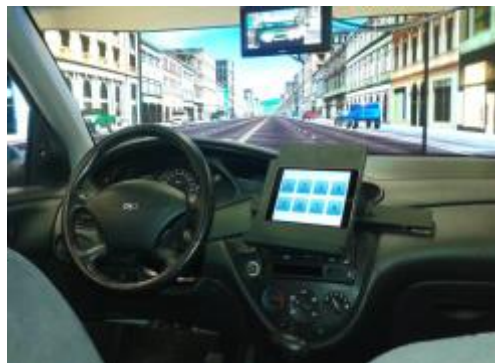
Figure 22. Driver's View of the Simulator with 10" Tablet
