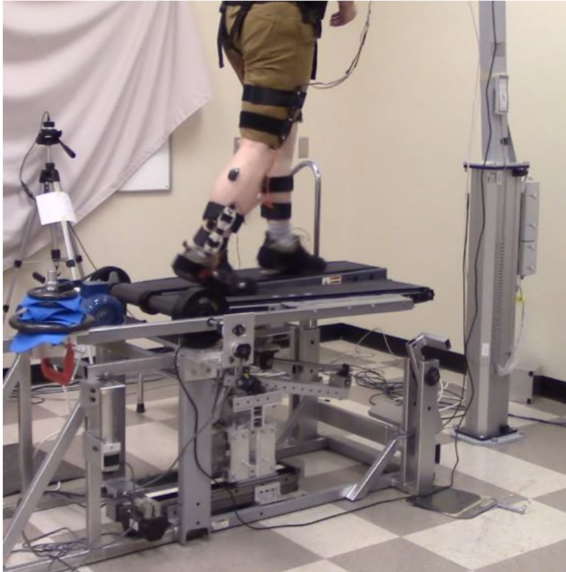
Figure 7.6: The subject experiencing a low stiffness perturbation to the right walking surface (Skidmore and Artemiadis (2016b), ©2016 IEEE).
