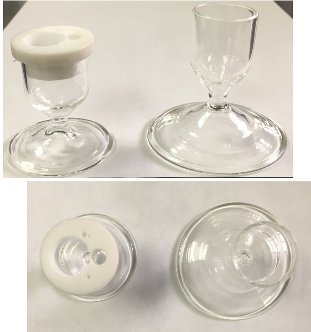
Figure A-1. Electrochemical cells for interrogation of proteins under diffusional conditions in small volumes of 0.5 to 5.0 mL.
