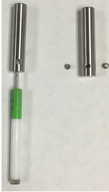
Figure A-5. Hardware to enable rotation with a standard disk electrode. The stainless steel adapter tightly holds the electrode via the two setscrews and allows rotation up to 4k rpm.
