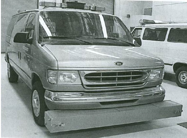
Figure 3.0.2 Profilometer used by the Arizona Department of Transportation to measure both roughness and rutting
