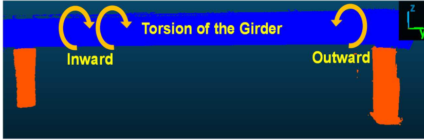
Figure 32. Classified Local Deformations of Highway Single-Pier Bridge 2
