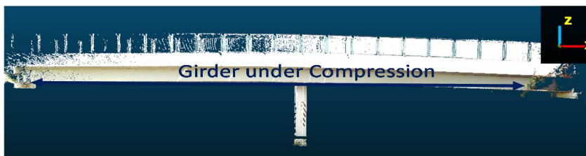
Figure 31. Classified Local Deformations of Highway Single-Pier Bridge 1
