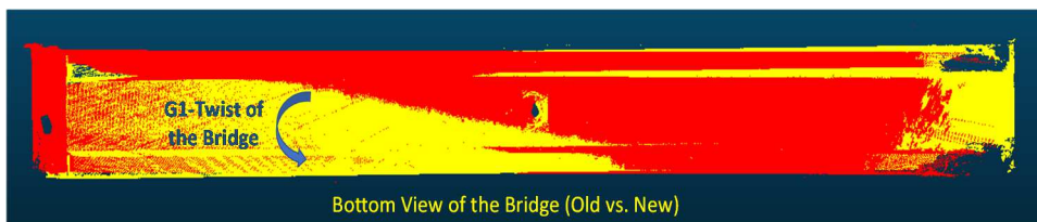
Figure 25. Detected global deviation (twist of the bridge)
