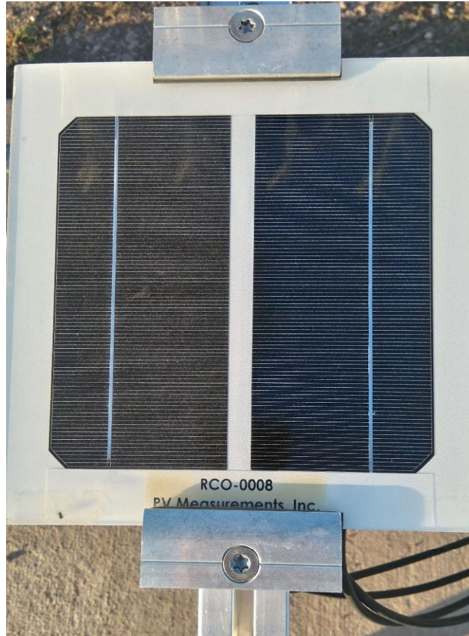
Fig 2.5: Sensor showing left half soiled and right half clean
