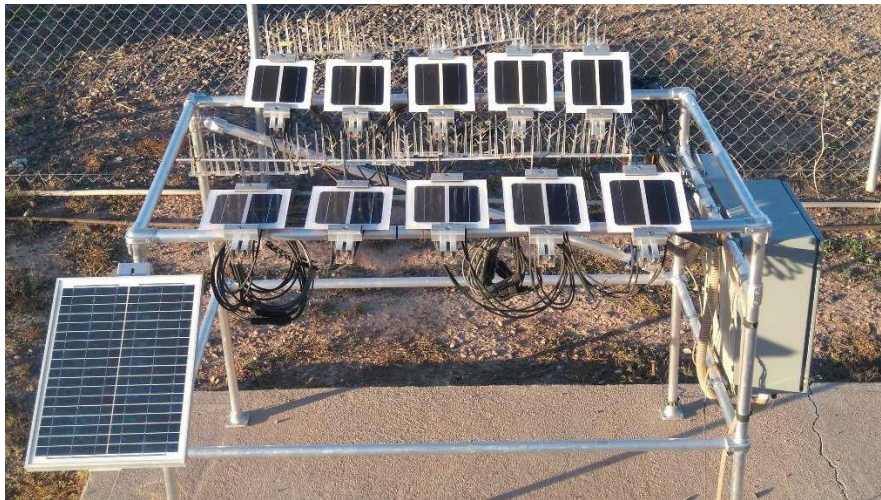
Fig 2.1: SANDIA soiling station located in outdoor testing field at ASU-PRL
