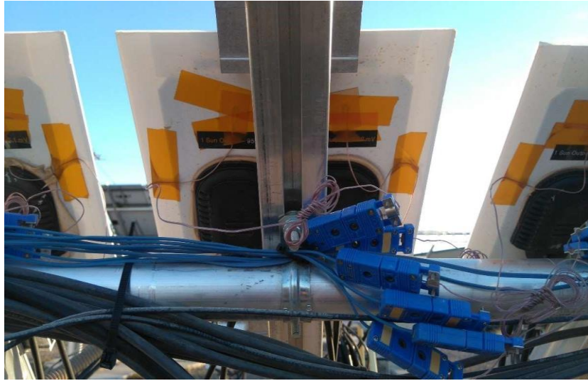
Fig 2.4: Back side of sensor showing attached thermocouples
