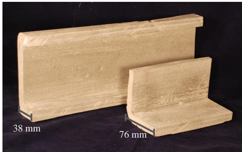
Figure 32: Pultruded TRC composite L and C structural sections
