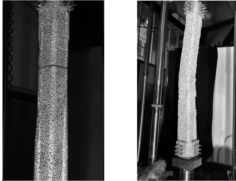
Figure 44: Tensile cracking and compressive buckling of 1.22 m long TRC L sections
