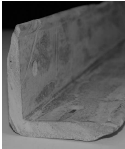
Figure 13: Cross section of pultruded TRC angle
