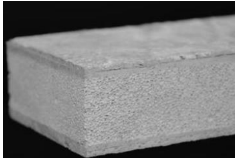
Figure 45: Pultruded TRC sandwich section
