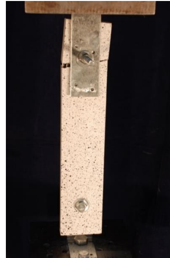
Figure 36: Replicate plot of ARG specimens tested in tension with bolted end connections
