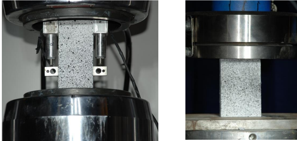
Figure 24: Direct tension and compression testing setup for pultruded TRC coupons with digital image correlation
