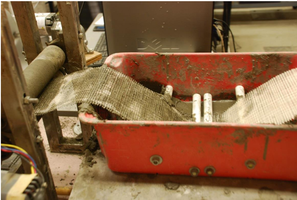
Figure 4: Coated textile leaving the paste bath and entering the DC powered rollers
