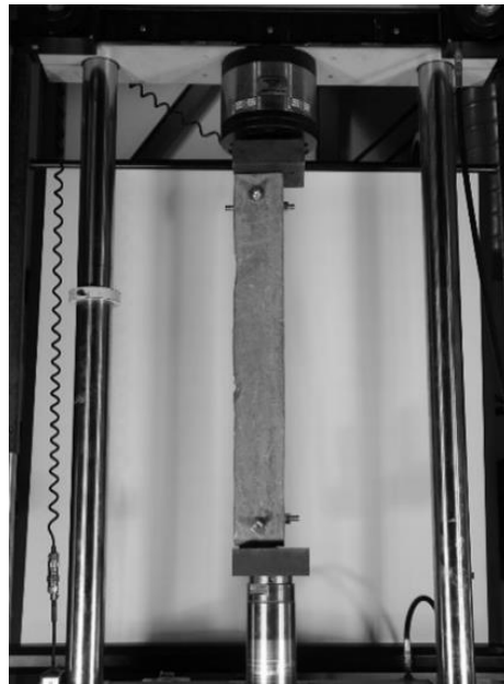
Figure 16: Tension testing setup of TRC angle on Instron load frame
