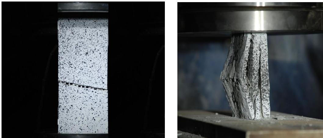
Figure 30: Tensile failure of ARG coupon showing single large crack along gage length and failure in compression displaying splintering and excessive delamination between all textile layers
