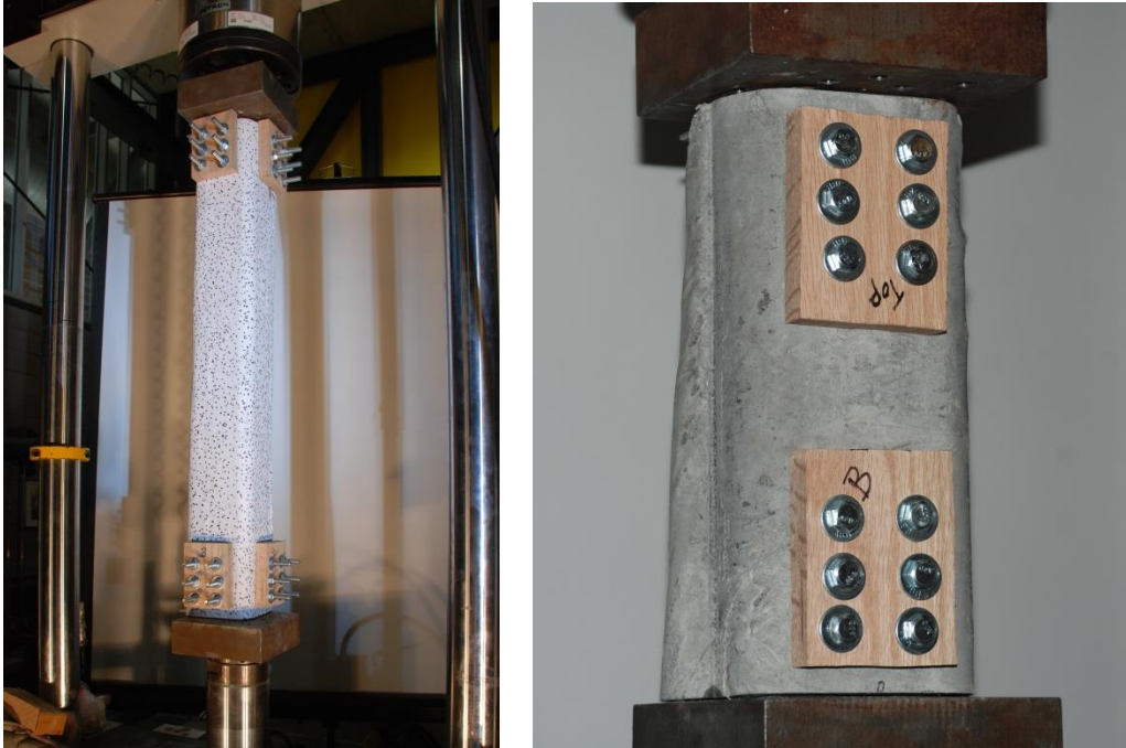
Figure 37: Tension test of full size TRC structural L-section and C-section with bolted connections on each leg
