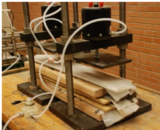
Figure 11: Pneumatic press before pressing a plate sample
