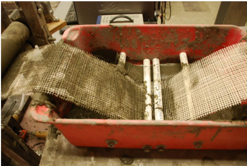
Figure 3: Textile passing through paste bath
