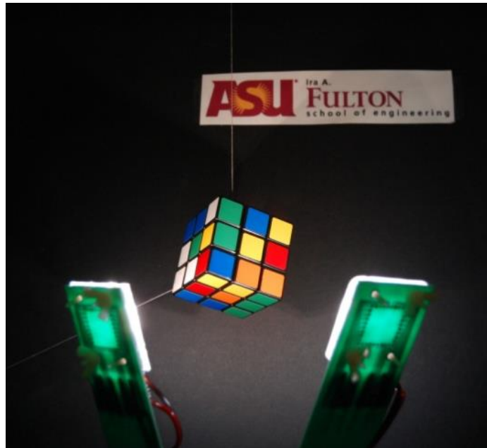
Figure 29. Performance characteristics of Pt 17 based WOLEDs using TAPC:PO15 as co-host materials. [a] Forward viewing external quantum efficiency (open squares) and power efficiency (filled squares) versus luminance of the WOLED. The device structure is ITO/PEDOT/NPD(30nm)/TAPC(10nm)/18%Pt-17:TAPC:PO15(25nm)/PO15(40nm)/LiF/Al. [b] An image of a magic cube illuminated by the WOLED demonstrating white color and high color rendering index value.
