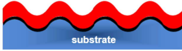
Figure 20. Schematic of film stack used to determine the unknown modulus of a thin film when the film of interest is not stable when directly deposited on the substrate material.
