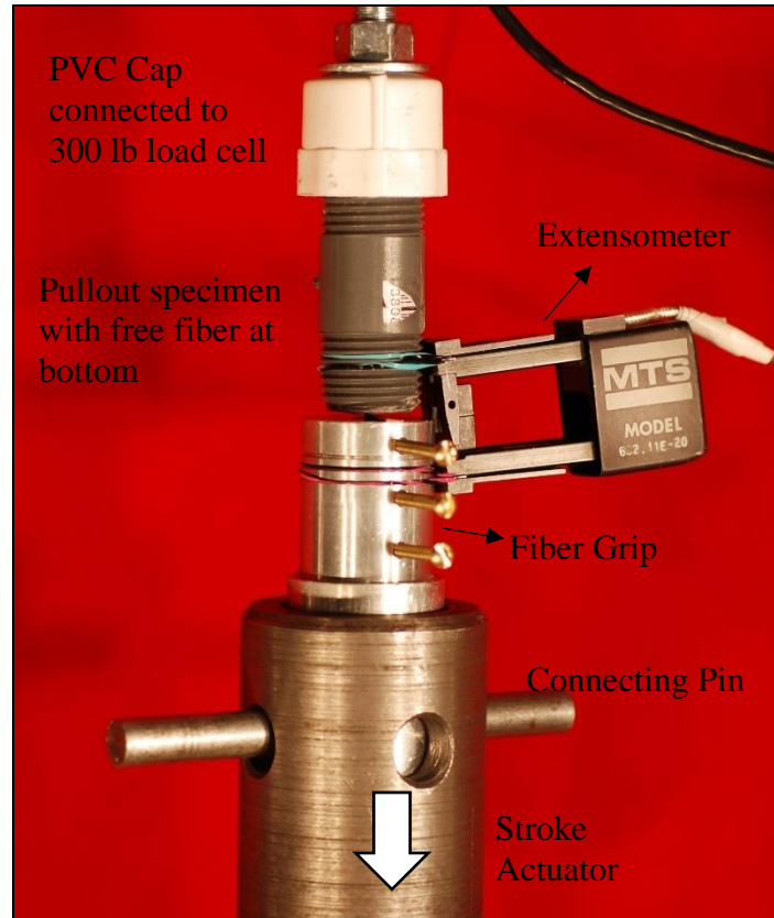
Figure 19. Test Setup for fiber pullout tests.
