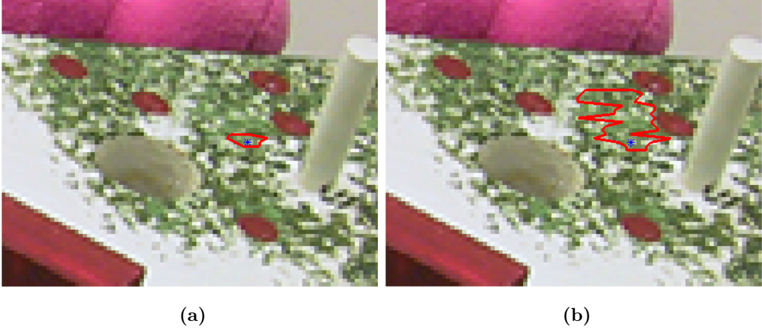
Fig. 4.3: The Boundary of the Support Region of a Considered Pixel (Blue Cross) in the Teddy Image is Shown by the Red Contour Surrounding That Pixel. (a) Original Cross-based Support Region [1] of a Pixel in the Teddy Image. (b) Modified Cross-based Support Region Generated by the Proposed Method of a Pixel in the Teddy Image.
