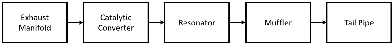
Figure 9: Typical Exhaust System Configuration
