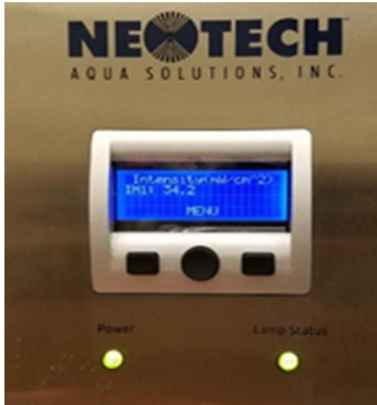
Figure 5. Close-Up View of Laboratory Scale UV Unit Control Box
