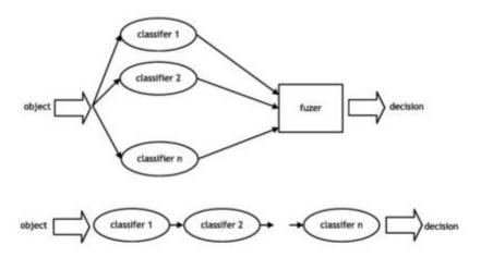
Figure 4: Parallel and Serial Topology of Multi-Classifier System [Woźniak et.al 2014]
