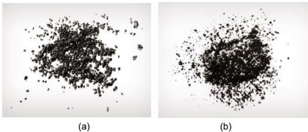
Figure 3. Photographs of a) GAC, b) PAC; from www.norit.com
