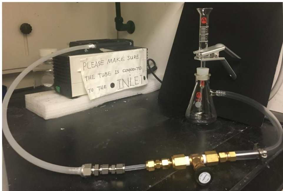
Figure 70. Photograph of the vacuum filtration setup at ASU.
