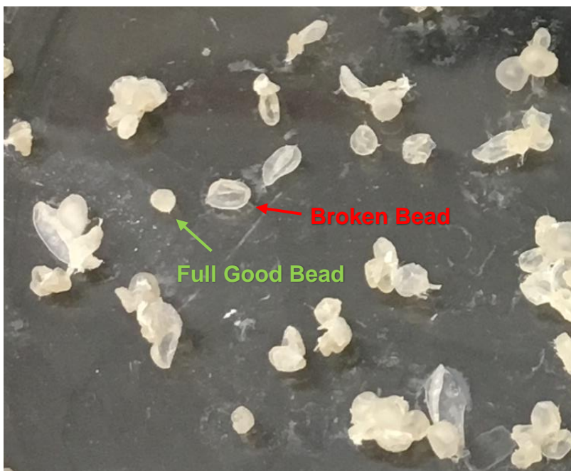
Figure 66. Picture of in-situ synthesized LDH/chitosan composite beads with 60% precursors as LDH part. Most of the beads were broken.
