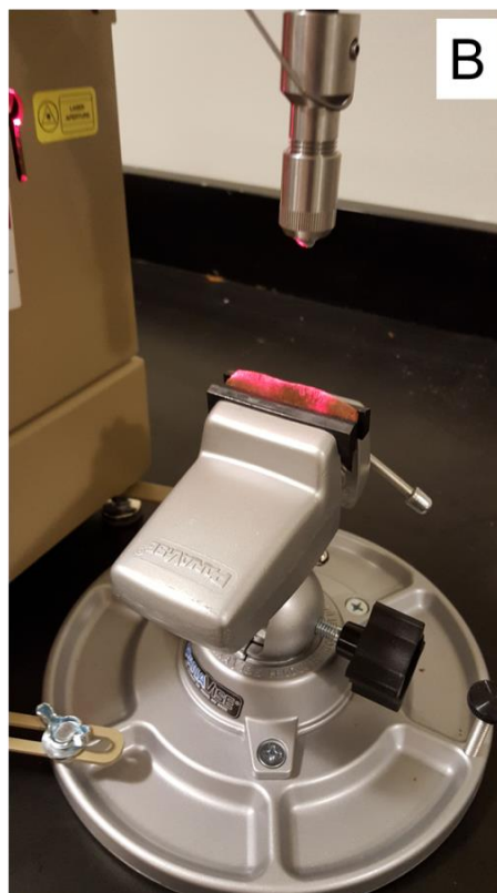
Figure 41. Taber Linear Abraser setup. A) Machine fully assembled. Note the horizontal arm with attached free-floating vertical boom with weights and abrasion tip on the right, B) Universal sample holder allowing for holding the stone tool with edge up. Note the red light, which is the guiding laser to allow for aligning the stone tool edge with the path of the abrader.
