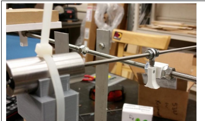
Fig. 15 3-D printed LVDT main body and core attachment with ball joint
