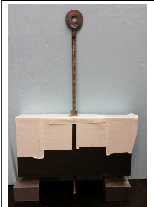
Fig. 12 Counterweight cup attached to vertical counterweight arm
