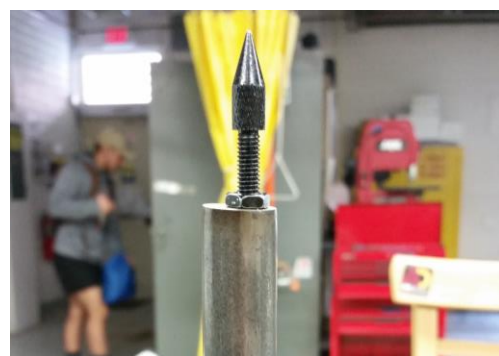
Fig. 13 Torsional arm pivot point attachment
