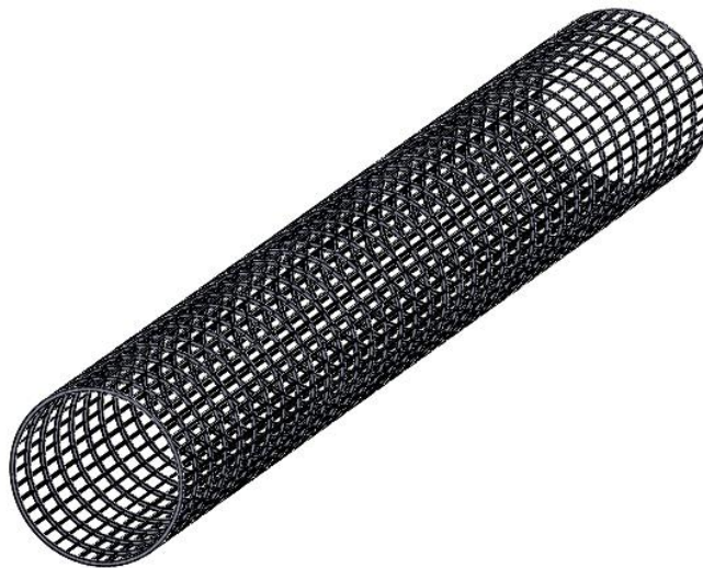
Figure 18. Business Jet: Full Fuselage Model without Skin
