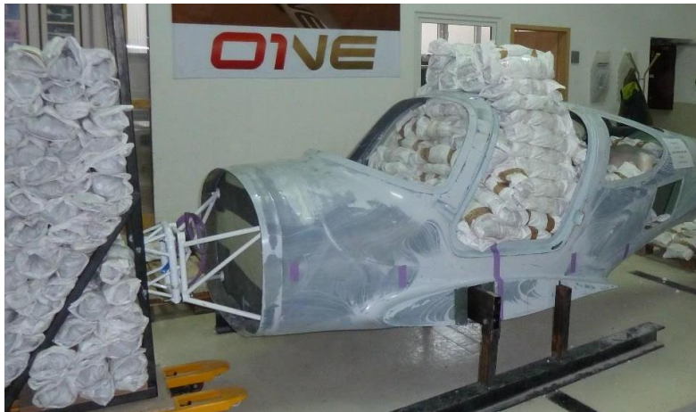
Figure 2. Example Structural Load Test. (2017, March 21). Retrieved from http://www.oneaircraft.com/static-testing-finished/
