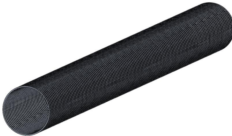
Figure 33. Wide Body: Full Fuselage Model without Skin
