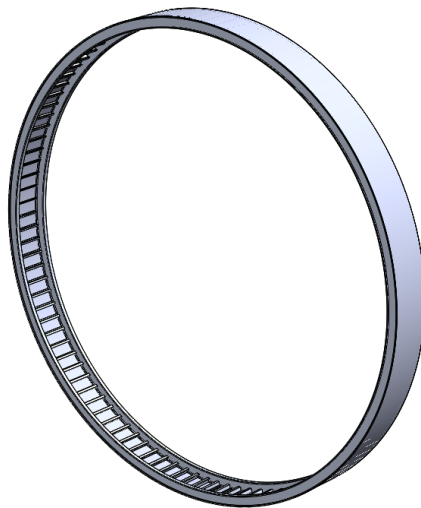
Figure 34. Wide Body: Single Fuselage Ring
