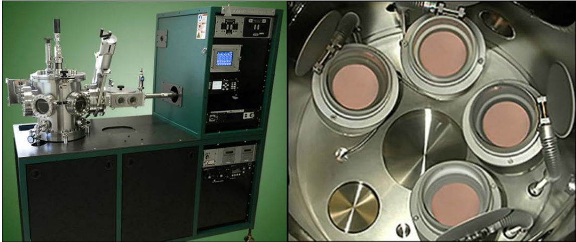
Figure 9: Left: Orion 5 Sputter Deposition Tool used to synthesize metallic and amorphous thin films. Right: Magnetron sputtering guns having copper targets. Pictures courtesy AJA International.
