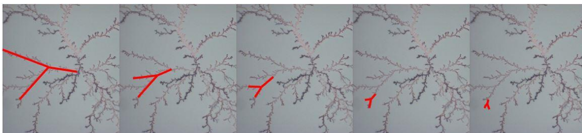
Figure 10: Five generations of self-similar Y-shaped elements in fractal Ag electrodeposit
