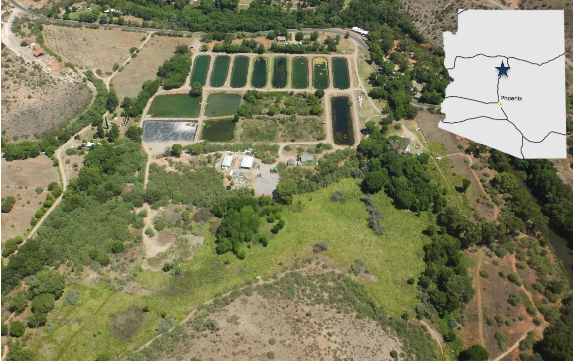
Figure 1. Bubbling Ponds Hatchery in Cornville, Arizona, looking north. Active fish-rearing ponds are the nine long oval ponds to the north and east. Fallow ponds are the four vegetated blocks in the south middle. The four ponds to the southeast were drained during much of the study (June 2015 – February 2016). The pond in the far southwest was lined with black polypropylene liner and remained empty. To the south of the managed ponds are a rocky ridge covered by trees and a wet meadow. Oak Creek borders the site on the east.
