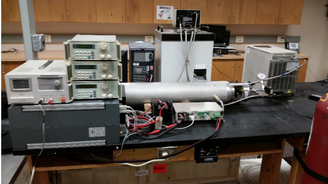
Figure 12: Bench Test Setup with the MH7000 tank.
