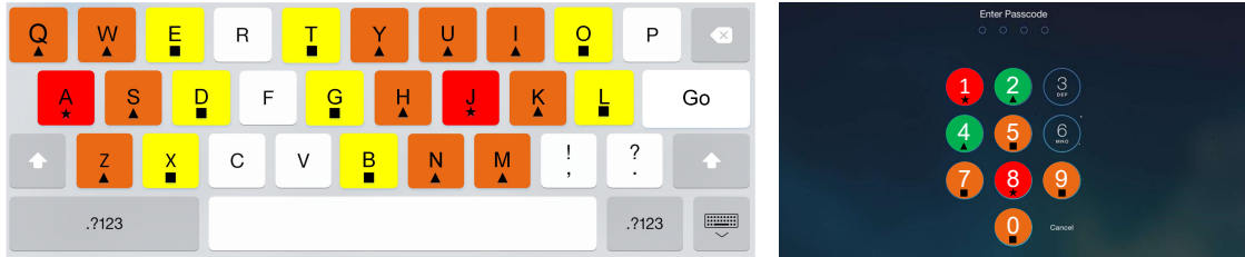
(a) One-hop and Two-hop Neighbors of Letters “a” and “j”. (b) One-hop Neighbors of Keys 1 and 8.
