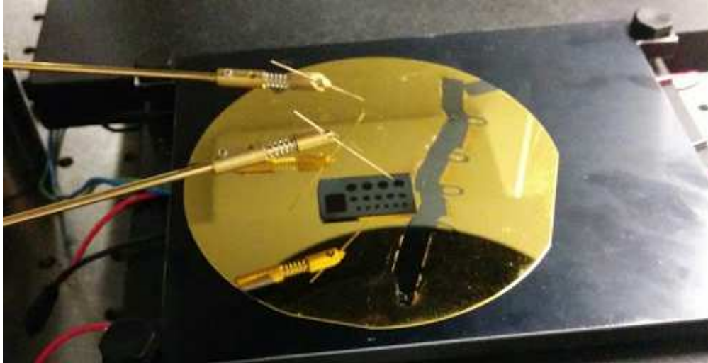
Fig. 5-8 Picture of the Monocrystalline Cdte/Mgcdte Double-Heterostructure Solar Cell and the Measurement Setup.
