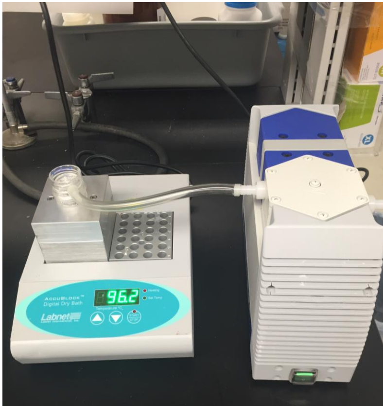
Figure 3.11 Agarose degassing system. 5 mL of agarose is dissolved by heating the solution at ~95°C in a 50 mL centrifuge tube with the standard cap attached, the falcon tube is removed several times for vortexing and placed back inside the heat block. The cap is then removed and a Millipore Steriflip unit is attached, an additional 50 mL centrifuge tube is attached to other side of the Steriflip (not shown) to create a seal and Tygon tubing is attached to both the Steriflip unit and the vacuum pump. The vacuum pump is then turned on for 5 seconds and then the agarose is harvested as described in (Conrad 2015).
