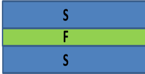
Figure 46. Cartoon showing grown S/F/S structures with S =Nb and F = Ni 80 Fe 20
