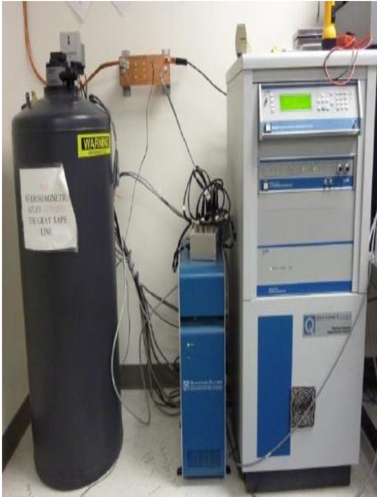
Figure 26. ASU-QD PPMS system for low temperature magnetic measurements
