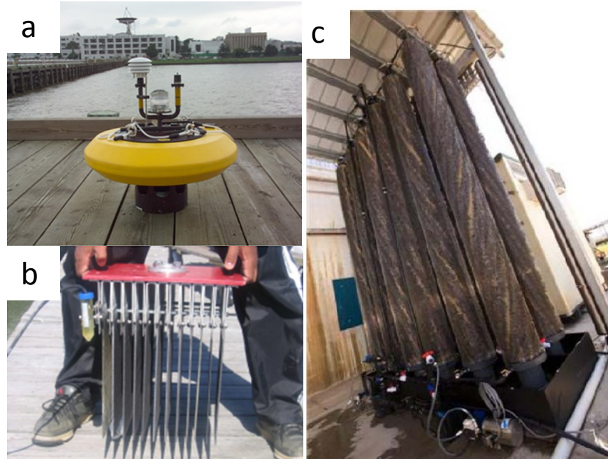
Figure 1.4. Photographs of various macroscale MFCs. (a) the first BMFC constructed by Tender et al. 2007, which has a mass of 230 kg, a volume of 1.3 m 3 and sustains 24 mW, (b) The second version of BMFC constructed by Tenders et al. 2007, which has a mass of 16 kg, a volume of 0.03 m 3 and sustains 36 mW, (c) macroscale MFC set up by the Advanced Water Management Center in University of Queensland, which has a volume of 1 m 3 with 12 modules.
