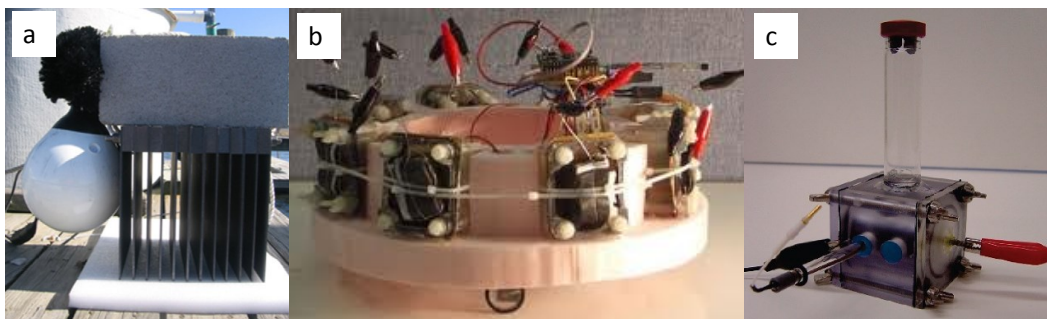
Figure 1.3. Photographs of MFCs for a variety of applications. (a) photograph of the first application of MFC as a viable power source to power a meteorological buoy, (b) robot with air-cathode MFCs on board, to perform sensing, information processing, communication and actuation when fed (amongst other substrates) with flies. This is the first robot in the world, to utilize unrefined substrate, oxygen from free air and exhibit four different types of behavior, (c) Single chamber MEC shown with gas collection tube (top), Ag/AgCl reference electrode (extending from the front), cathode connection (left clip) and brush anode connection (right clip).
