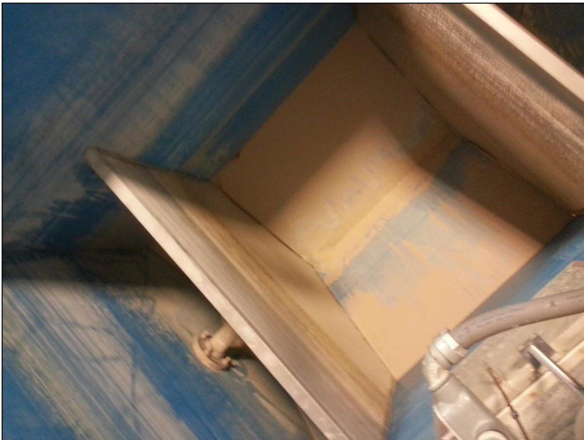
Figure 6: Large basin/water reservoir at the downstream terminus of the flume. Here the basin was drained to allow cleaning of the relatively small amounts of sand and silt deposited after many erosion experiments.
