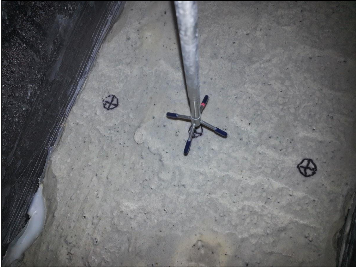
Figure 13: Vectrino probe and pre-determined points of interest to measure flow data. In this case, the flow was to be measured and compared across the width of the flume.
