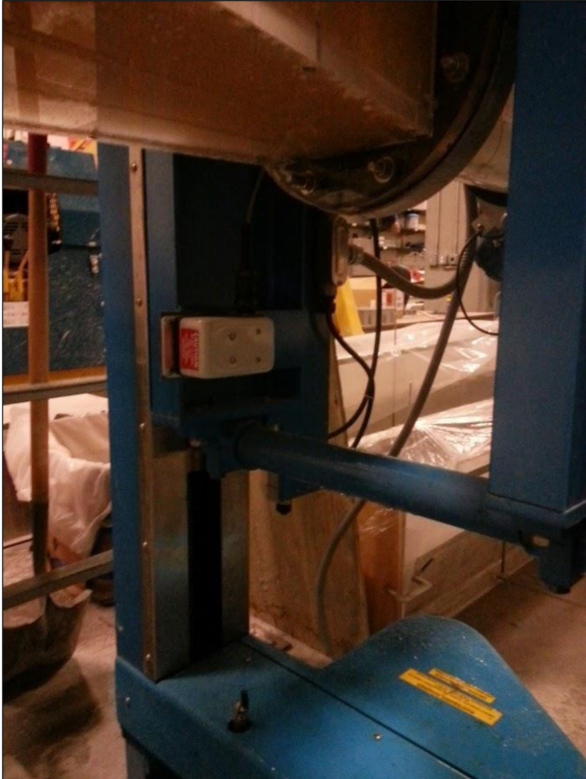
Figure 7: Screw drives that control bed slope of the entire flume (opposite end is hinged). In the background are future inserts containing concrete in the process of curing.
