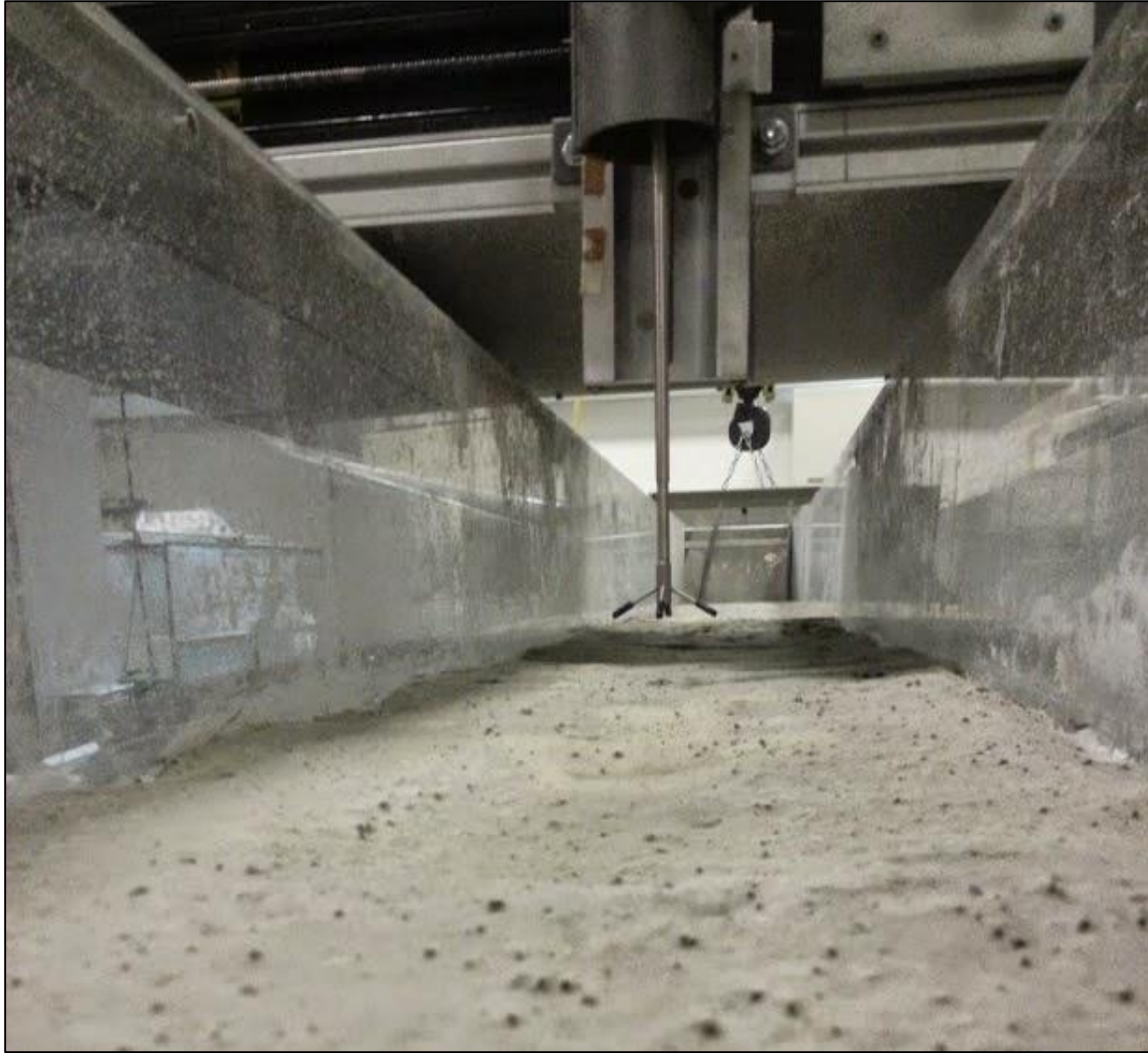
Figure 12: Vectrino probe in place above the bed surface. Distance to the bed is manually measured from the concrete surface to the central head of the probe. Holding the Vectrino is a precise screw-drive mount, and that is attached to the scanning laser cart.
