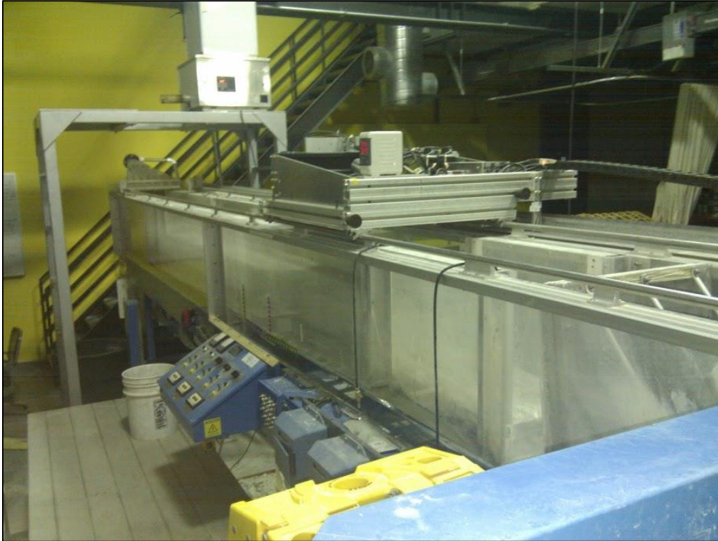
Figure 8: Flume control area. Reservoir basin is blue object on bottom-right, scanning laser is attached to cart sitting atop the rails halfway upstream flume, control panel is blue object just below the cart.
