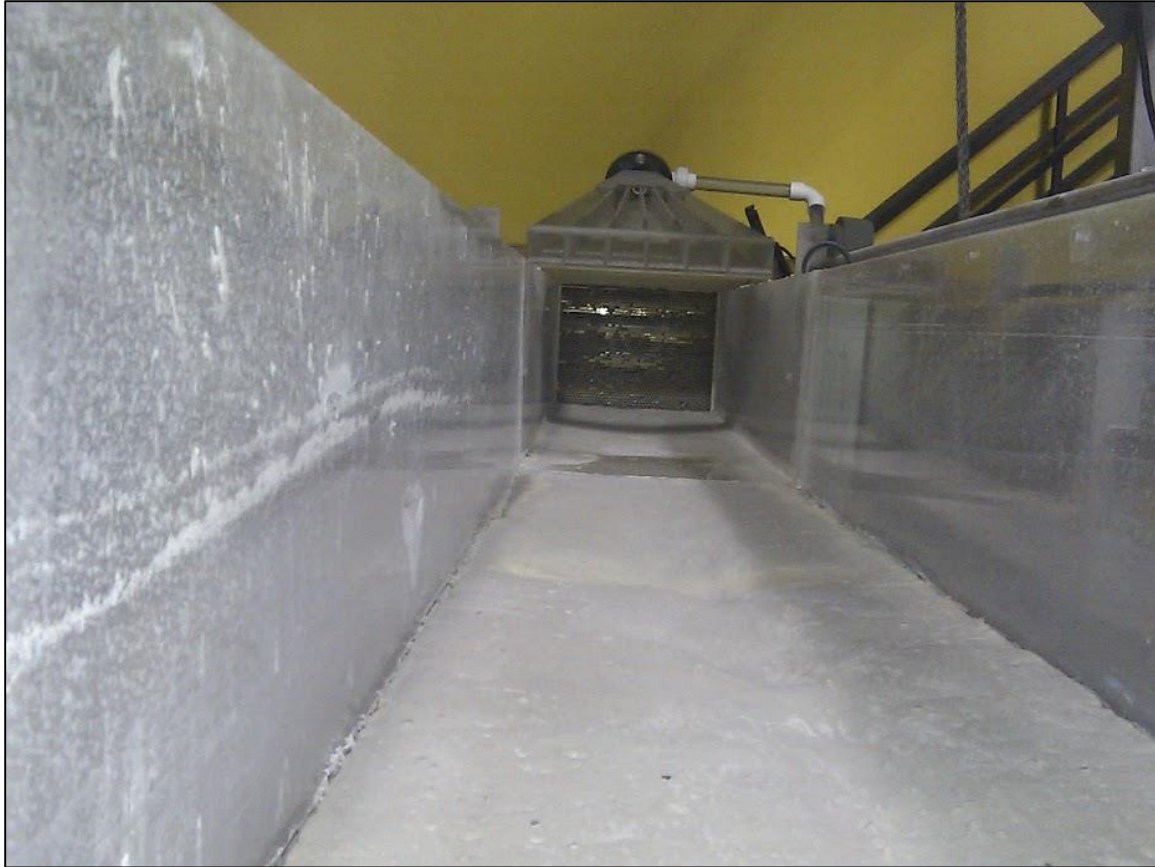
Figure 5: Upstream section of flume, including honeycomb flow gate (far background), followed by the transition insert, and nearest the concrete insert (semi-smooth roughness seen here). Above the flume at the most upstream section is the suspended sediment fan.
