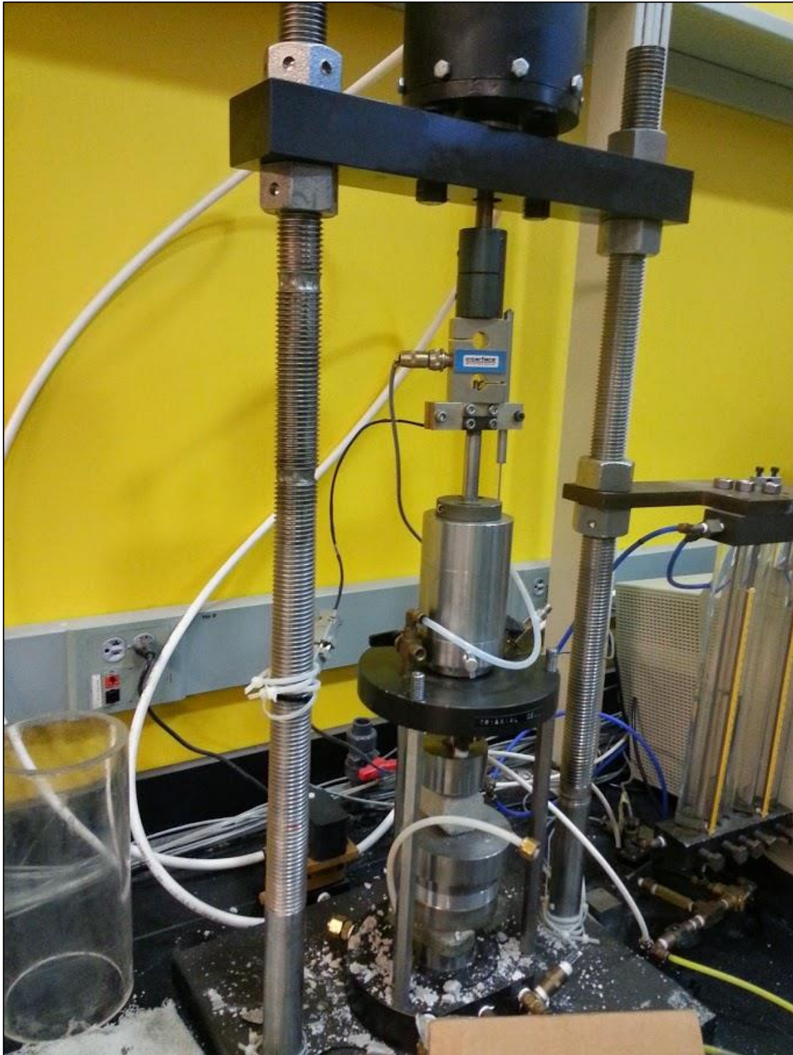
Figure 10: Equipment used for Brazil test method of measuring tensile strength of concrete test samples.
