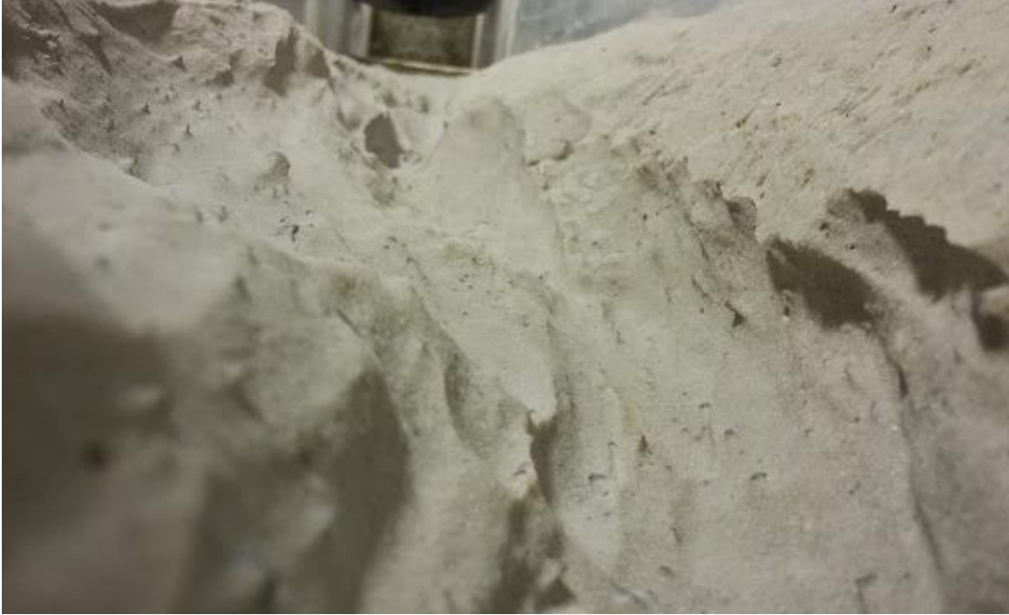
Figure 48: Sharp erosional facets created from repeated erosion experiments using smallest sediment ( D_{50} = 0.56 mm), which hovers near the transition between suspended and saltation transport modes.
