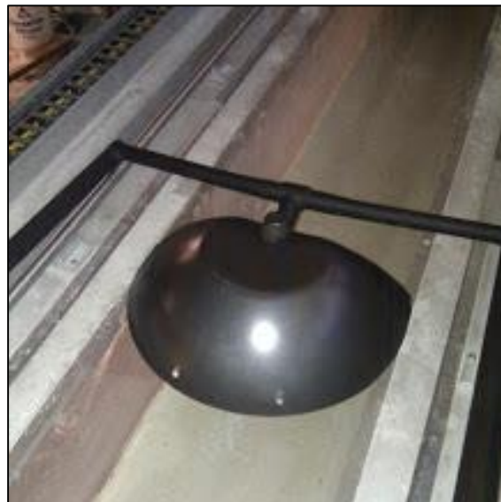
Figure 9: Sediment disperser placed below sediment hopper used to evenly distribute sediment grains along width of the flume insert.
