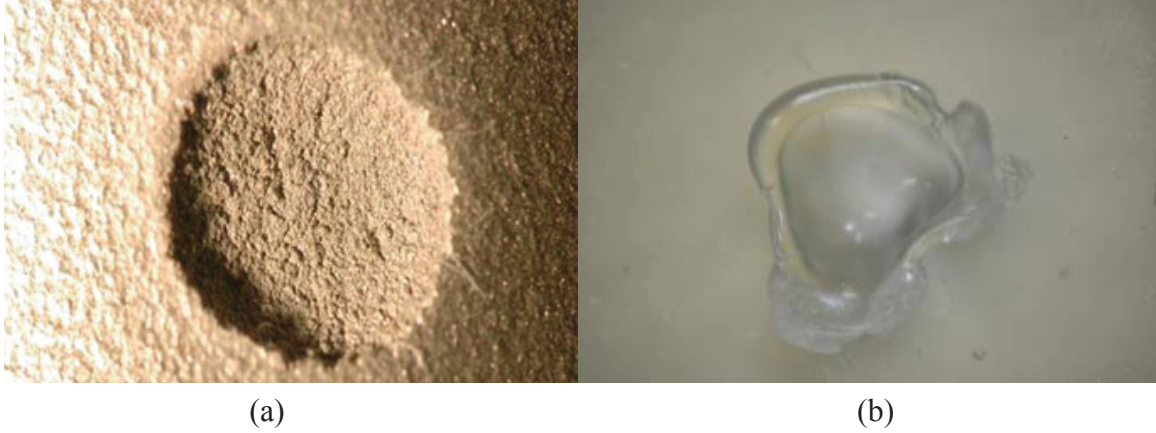
Figure 2.5: Typical cavitation erosion pattern induced by cavitation erosion on (a) metal and (b) polyurea surfaces [68].
