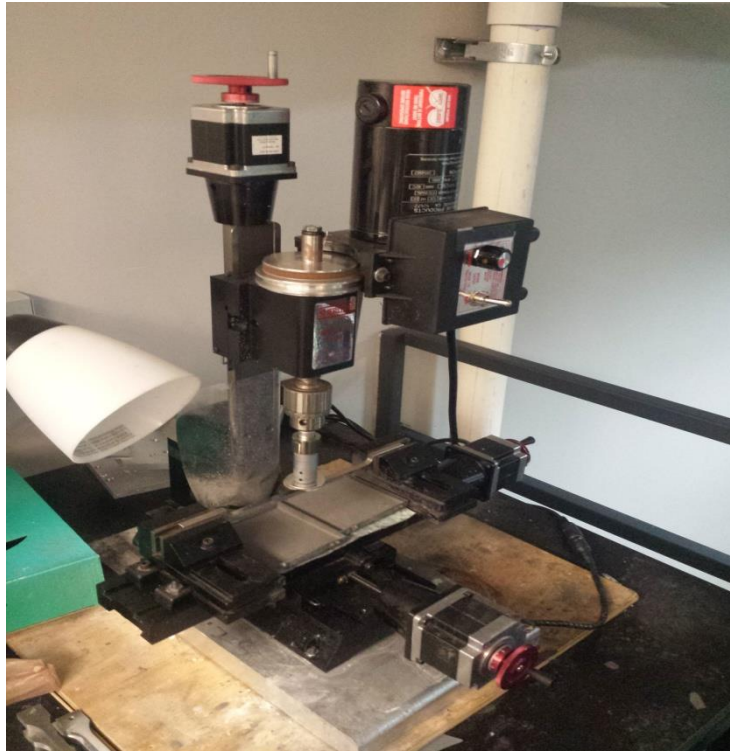
Figure 41. CNC machine for polishing samples.
