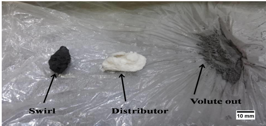
Figure 52. Examples of debris specimens provided by AORA: Swirl, Distributor, and Volute out.
