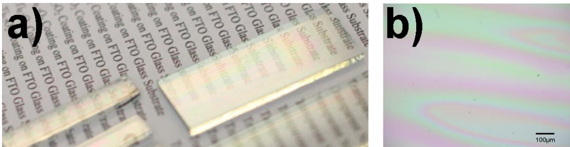
Figure 14. a) Photographs of transparent nanoporous Zr-doped TiO 2 films on conducting glass substrates, and b) the color variation caused by slight thickness variations, seen under an optical microscope (scale bar = 100 μm).
