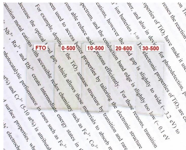
Figure 46. Photograph of plain FTO glass and FTO glass with thin films of 0-500, 10-500, 20-600 and 30-500 appearing from left to right.
