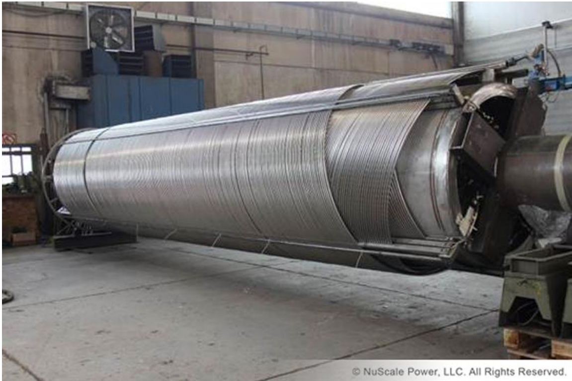
Figure 1.4 Photo of NuScale full-length helical coil steam generator [32].
