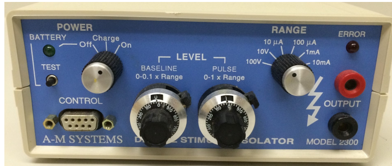
Figure 5.3: Front view of the digital stimulus isolator from A-M Systems. The current and voltage levels must be manually selected using the corresponding knobs.
