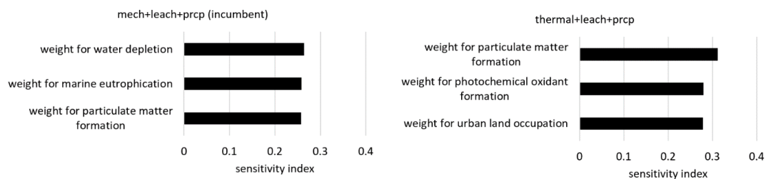
Figure 27 Global sensitivity analysis results (with weights). Global sensitivity analysis results showing the values of the sensitivity indices for the three most significant input parameters (out of a total of 144 input parameters). The environmental ranking of the incumbent “mech+leach+prcp” (left) and the novel “thermal+leach+prcp” (right) recycling alternatives are most sensitive to the weights assigned to the three environmental impact categories.
