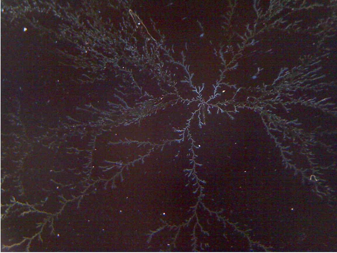
Figure 4.1: “Low field” physical sample at minimum magnification. Approximately 1cm wide, grown for 4000s with an applied bias of 10V.
