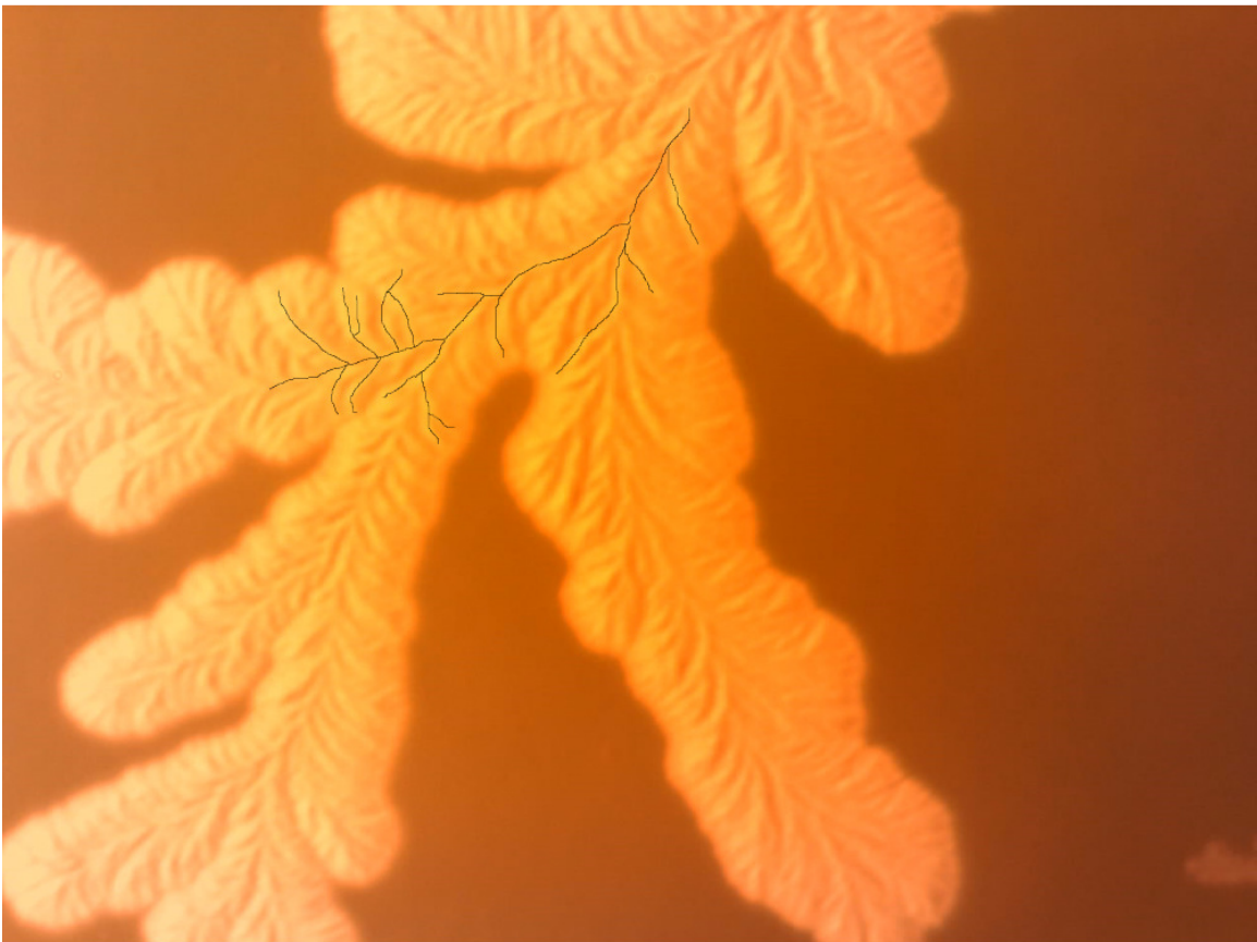
Figure 1.1: Magnified view of a dendrite sample showing fractal patterning. A small extent of the branches inside a major arm is traced in black to highlight the similar bifurcation occurring at smaller scales.
