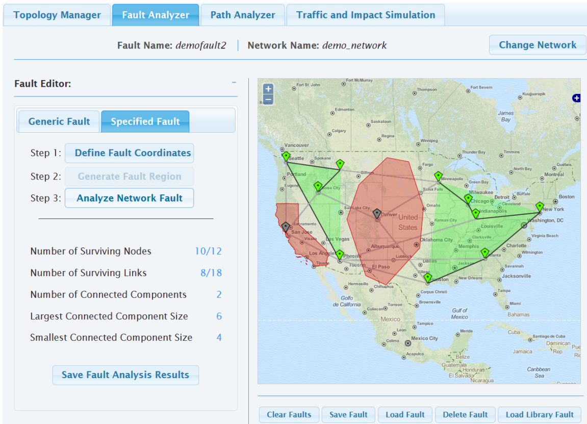
Figure 21: Fault Analyzer – Fault impact of the user specified fault and an imported library fault (coordinates for the state of California, USA)
