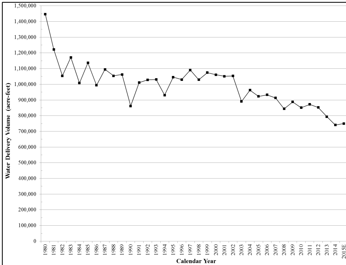
Figure F1. History of SRP Water Deliveries. The ResSim model was built per the 2003-2011 average delivery (900,000 acre-feet/year). (data courtesy of SRP)
