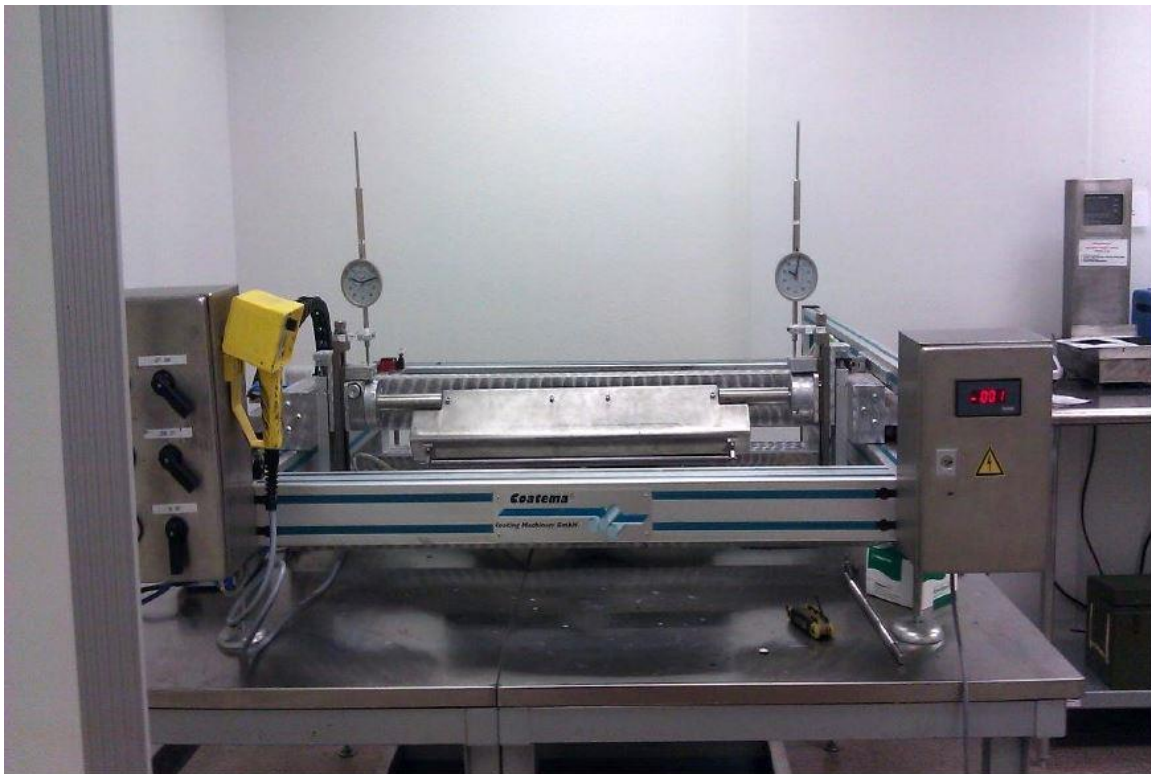
Figure 11 Easycoater Equipment (EC26, Coatema) Used for Coating GDL
